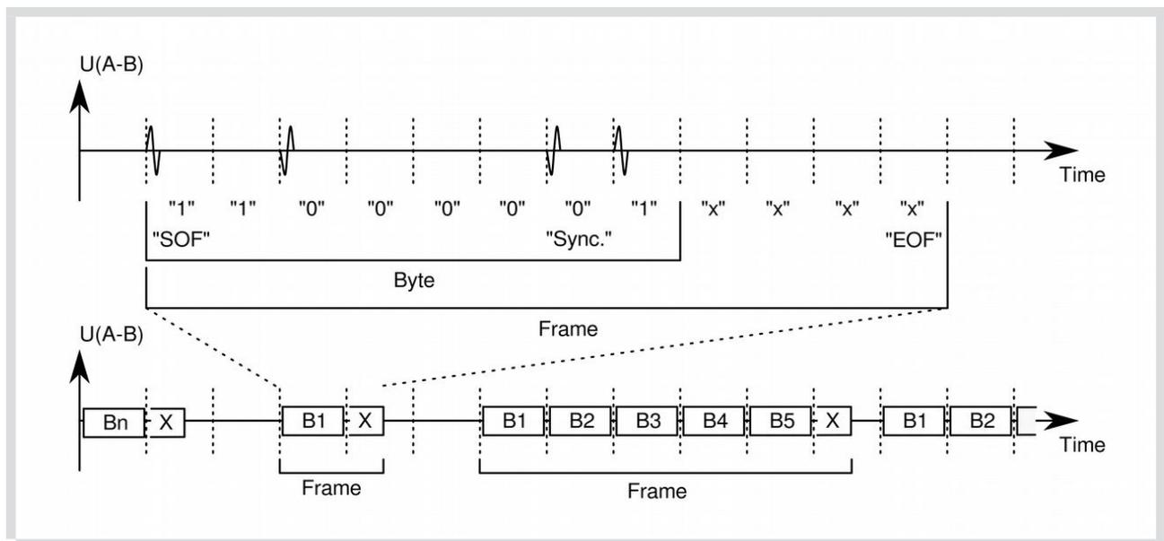
Partially transmitted Byte **X** must be discarded because it contains no data. Before ending the transmission with EOF, multiple Bytes can be transmitted in tight sequences. The Bytes transferred together will behave as a single stream of bits and there is no need to transmit a pulse at the beginning of every following byte.
