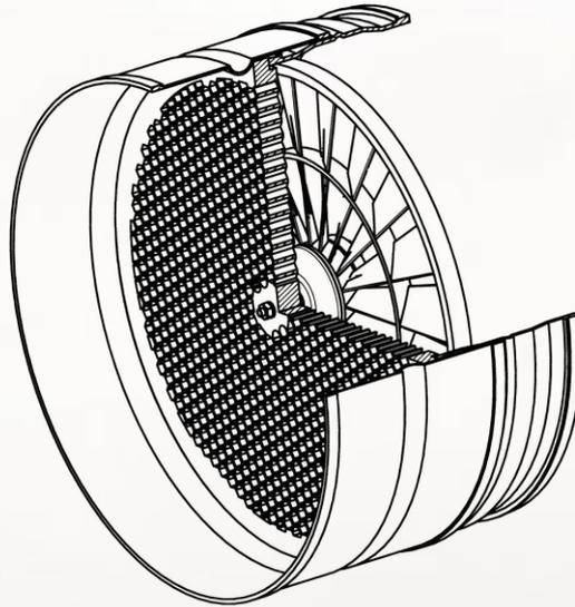
The InFlow Anemometer is an air-flow measurement device installed stationary into the building management system. It measures the airflow continuously over time. The measurement results are provided periodically with a period of 1–2 seconds. The following data is provided:
