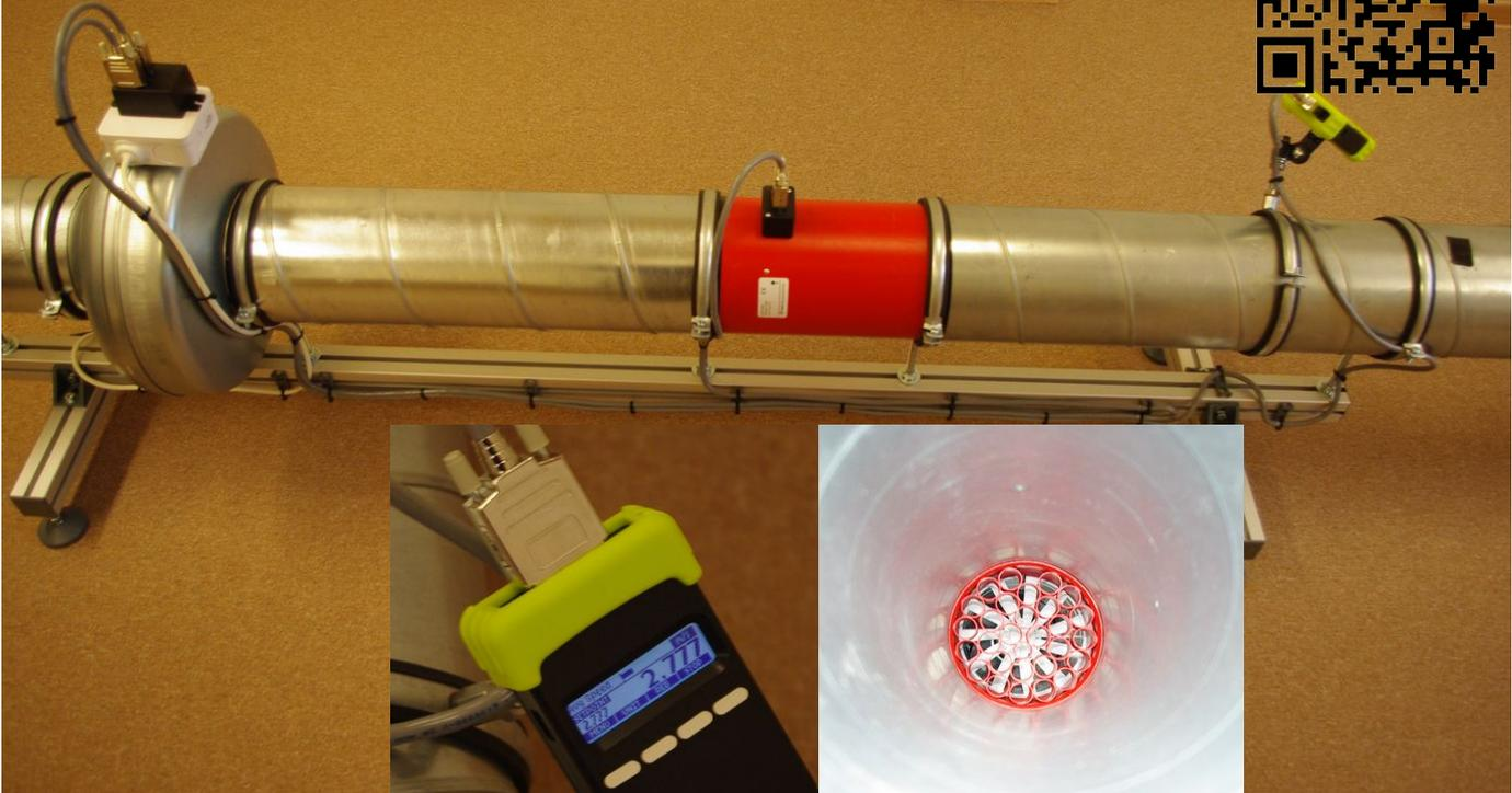
This is air-flow reference measure device. It keeps steady airflow through the tunnel and updates the flow-rate 2 times in second. Value is shown on graphical LCD display with back-light. With this device you can:
