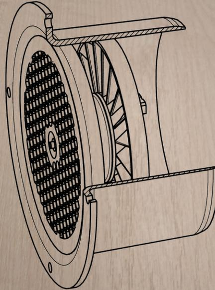
The Fresh Air Anemometer is an air-flow measurement device installed stationary into the building management system. It measures the airflow continuously over time. The measurement results are provided periodically with a period of 1–2 seconds. The following data is provided:
