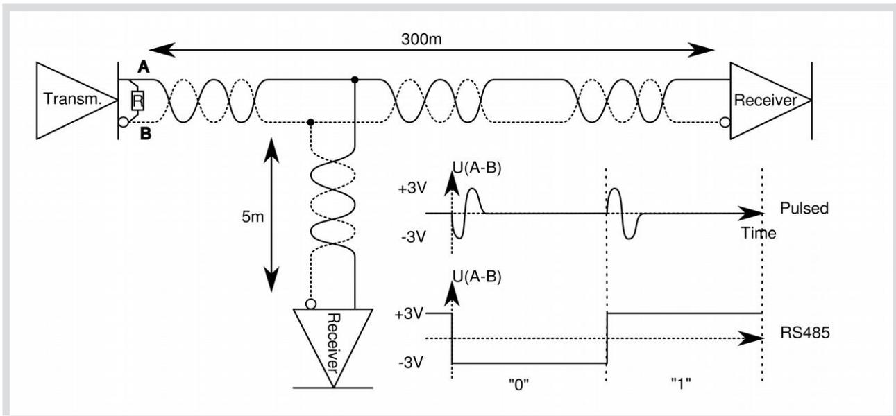
Most of the time, the messaging bus would not be powered in state "n" contrary to the existing systems. Therefore, less energy is spent for the data transmission. The transmitter and the receiver can be designed to consume energy only when the short pulse is transferred.
